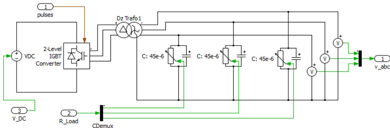
Fig. 5. The PLECS circuit model of the inverter, the transformer, and the output LC filter used in the simulations.
