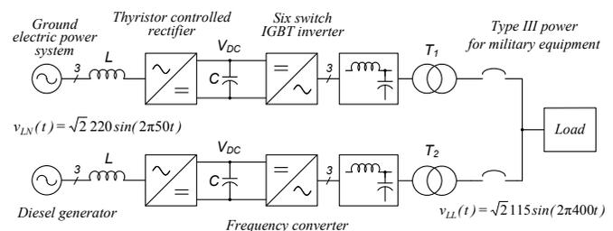
Fig. 1. The single line diagram of a ground electric power interface system including two parallel connected 400 Hz frequency converters.
