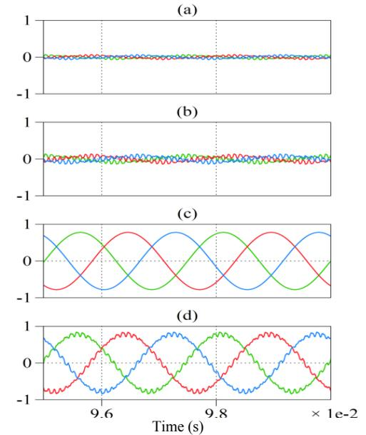
Fig. 4. The simulated waveforms of proposed control system: (a) the signals coming into and (b) the signals generated by the PI controller4; (c) output of the outer voltage loop and (d) the modulating control signals for each phase.
