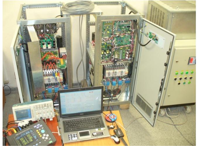
Fig. 6. The experimental step up for two 10 kVA parallel connected frequency converters.
