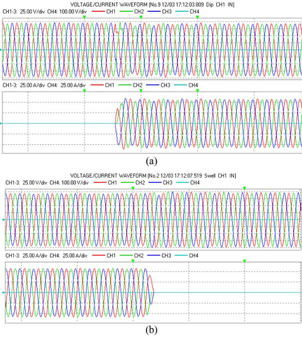
Fig. 8. The three-phase voltages and currents: (a) when the load is applied, (b) when the load is removed.
