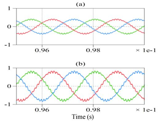
Fig. 3. The simulated waveforms of classical control system: (a) the signals coming into and (b) the signals generated the PI controller2.
