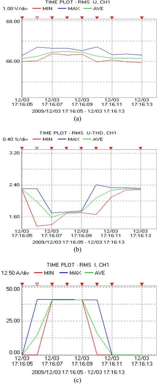
Fig. 9. The PQ meter recordings during a dynamic response test: (a) the profile of the RMS output voltage for one phase, (b) THD of the voltage for the same phase, and (c) the RMS current.
