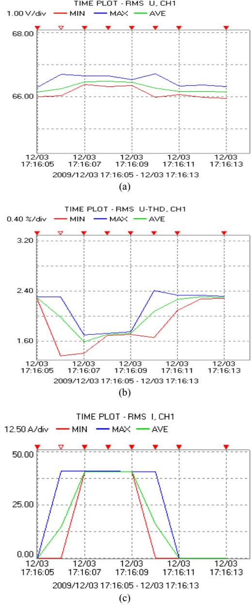
Fig. 9. The PQ meter recordings during a dynamic response test: (a) the profile of the RMS output voltage for one phase, (b) THD of the voltage for the same phase, and (c) the RMS current.
