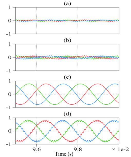
Fig. 4. The simulated waveforms of proposed control system: (a) the signals coming into and (b) the signals generated by the PI controller4; (c) output of the outer voltage loop and (d) the modulating control signals for each phase.
