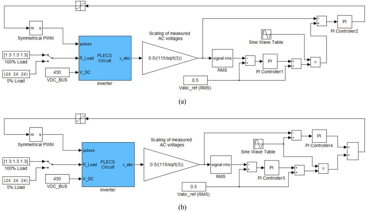
Fig. 2. The Simulink model of the control system: (a) the classical SPWM method and (b) the improved SPWM controller.
