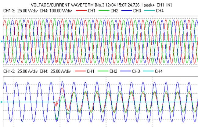
Fig. 10. The voltages (upper trace) and the currents (lower trace) when slave unit is energized while the master is supplying the full load. The CH1 is the slave current, CH2 is the master current, and CH3 is the total load current.
